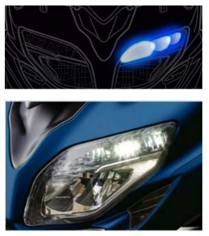
Activation of additional lighting units to illuminate the bending road
