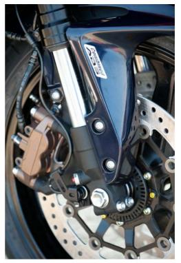
Front wheel disk brake fitted with ABS
